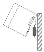
Start at the outer left location with the installation of your head module and install the peripheral modules to the right of this.
